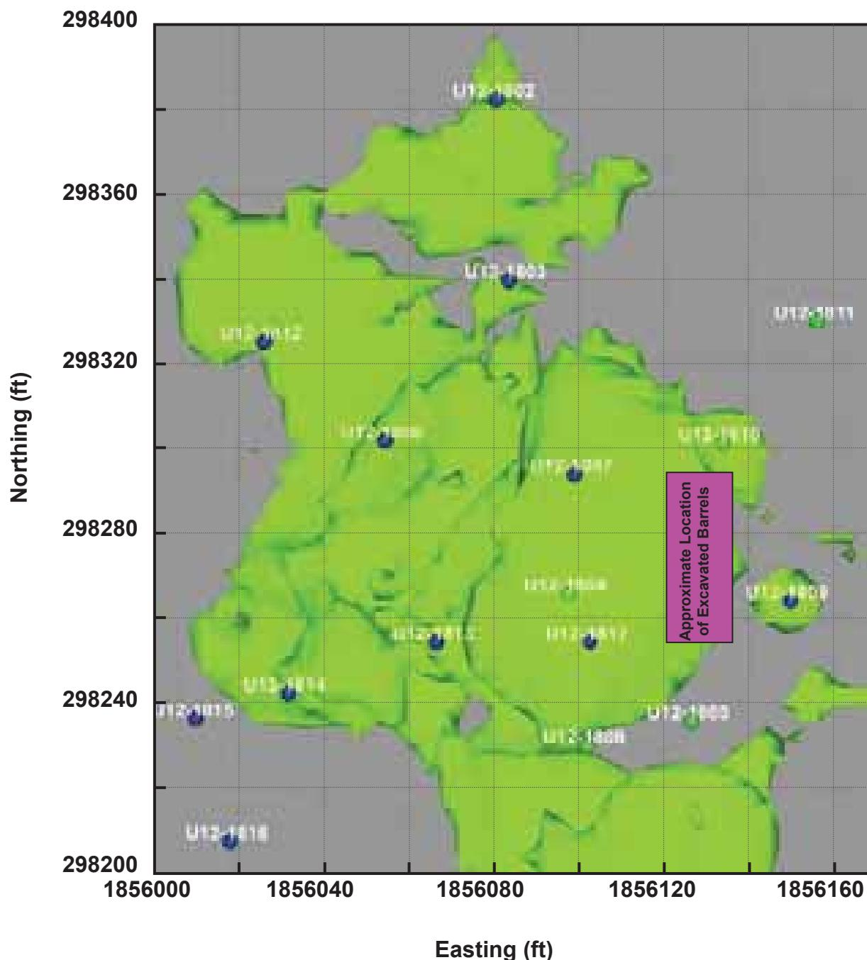
Figure 5-9. Final model of TCE contamination in soil, 100 µg/kg iso-concentration surface, constructed using 599 wireline soil samples from 16 borings.
